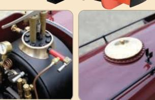
feed pumps, coal fired copper boiler, displacement lubricator, water and pressure gauges, etc. Alice will pull up to four adults on level track and is as capable and characterful as her full size counterparts.
