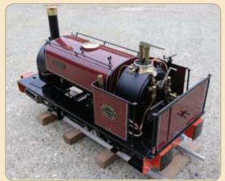
Stephensons link valve gear with cab reverser, screw down brake gear, hand and axle boiler
