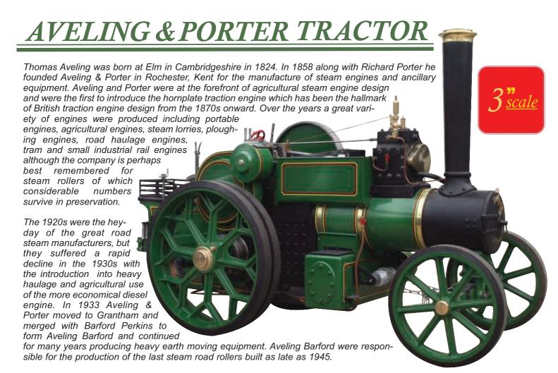
THE MODEL is based on the G.N.D 4hp Tractor of the 1920s and features a 6" dia copper boiler, silver soldered throughout (complete with test certificate). Water is held in the tender and belly-tank and fed to the boiler via a crankshaft pump, with an injector available as a optional extra. Steering is by worm and wheel via chain to the front axle. The full length canopy (optional) can be removed to facilitate driving.
