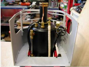
doing any assembly or cab shell on the chassis This was fine but it is around the boiler, no There was one problem, provision to hold the cab presume that it should the force of gravity, not a working model so a were drilled in the cab corresponding 3mm put in the top of the
