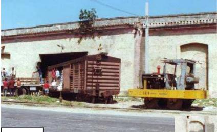
The little engine shown in Figure 20 was shunting the freight line at Cardenas. It shows just how lose a chain drive can be, and still work.
