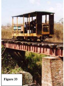
The last word in rail cars comes from Pepito Tey Mill and runs on 2 ft 6" gauge. It is fitted with a single driven axle at the front and a bogie at the rear, not an object of great beauty but it does the job. Figure 33.
