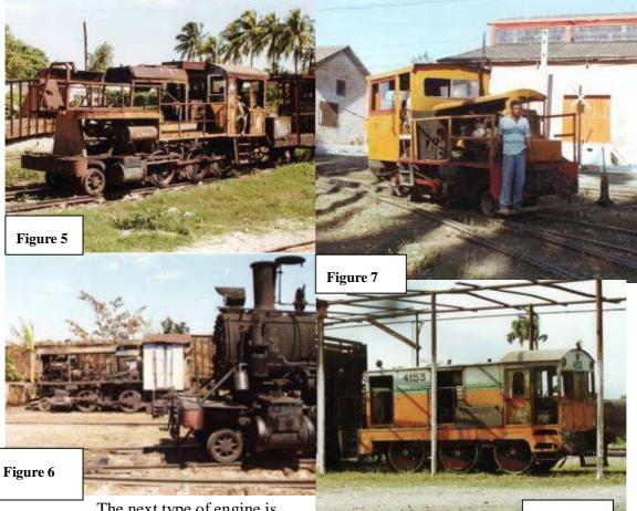
The next type of engine is even more unusual, steam engines converted to diesel.
