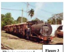
fireless engine. This is composed of the largest boiler the loading gauge will
