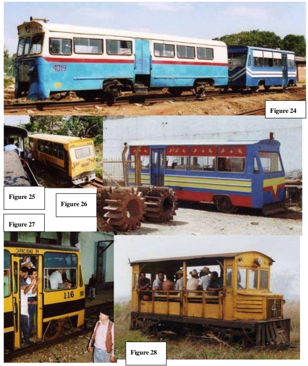
The first railcar seen in figure 24 is typical of many different one off types, most four wheelers have the long overhang at the front as seen on this example. The second railcar
