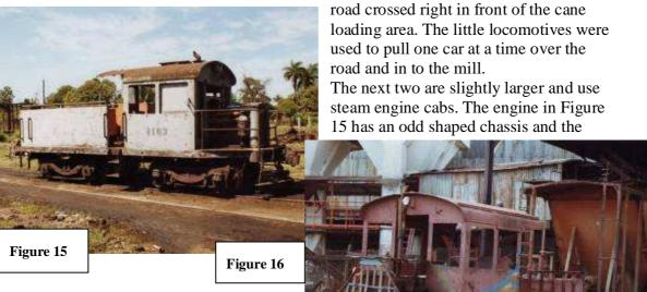
bogies are also unusual, perhaps an old tender chassis. This is also the only railway locomotive I have ever seen bump started. This was done from the back with a tractor equipped with a pusher plate! Figure 16 shows an engine with a similar
