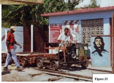
Passenger railcars come in all shapes and sizes, it is a job to know which are home made and which are commercially produced. Here are some four wheel examples.
