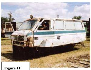
other has just a single front wheel. Both boast the original steering wheel in place, presumably for the hand controls. The original petrol engines are now long gone, replaced with a Russian diesel engine probably from a tractor.
