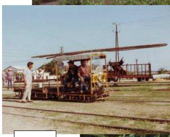
Speeders area familiar part of the Cuban railway scene. They are mostly powered by a Russian twin horizontally opposed motorcycle engine. Their main use is for track maintenance gang transport but they are also sometimes found on local passenger trips. They usually live on a short length of track laid at right angles to the main line, and are manhandled on to the track when required.
