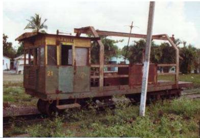
Figure 21 is a powered track maintanace car on Hermanos Ameijeiras mill, 3 ft gauge. This is a straight freight car conversion and looked to be out of use though it is sometimes difficult to tell. It is amazing what can be achieved with a battery and a can of fuel.
